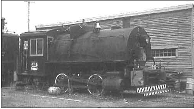
The CRHA's first steam locomotive was E.B. Eddy number 2, this 0-4-0T was built by Montreal Locomotive Works in 1925 and was stored at G.M. Gest's Construction Company premises in Dorval until it could be accommodated at the museum. CRHA Archives, Fond Angus # 3992.
