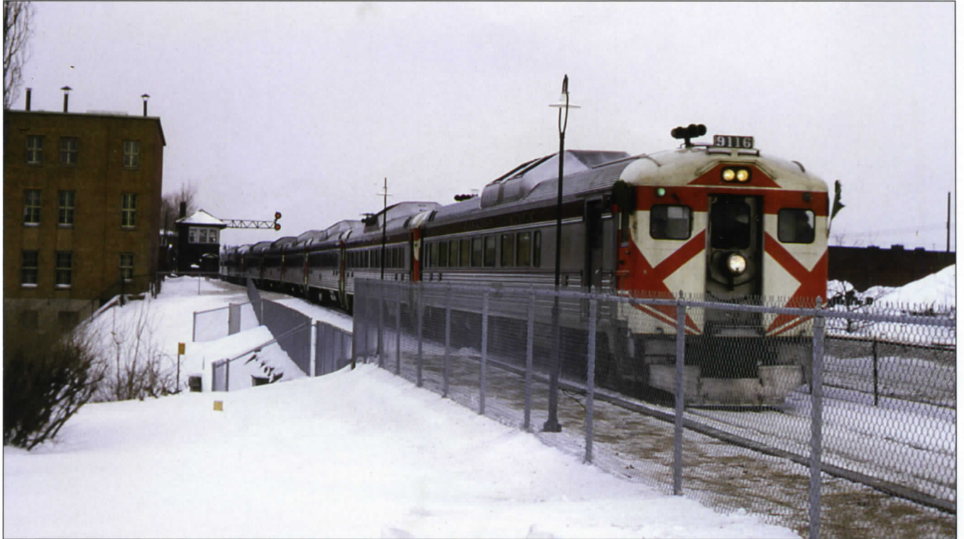
On Christmas Eve 1968, ex Leigh Valley 9116 leads CPR Commuter Train First 243 sporting the green flags indicating a second section to follow as per rule 21 of the Uniform Code of Operating Rules. Noteworthy is the fact that no less than twelve RDCs are in the train's consist. Early dismissal of downtown Montreal office workers at noon on Christmas Eve, required the use of the record twelve RDC's on train 243. The photo was taken just east of Westmount station. CRHA Archives, Fond Angus # 8414.
