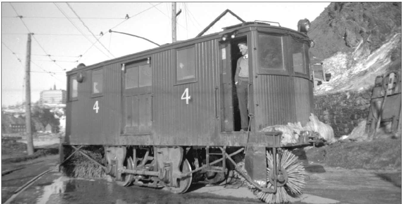
This double-truck sweeper (second #4 as first destroyed in 1921 fire) was acquired new in 1922 from the Russell Car & Snowplough Co. in Ridgeway, Penn. The sweeper is posing in front of the company's St. Laurent Street car barn in Lévis which opened in 1924. Al Paterson Collection
