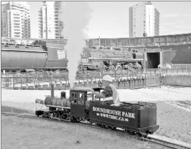
The “Sweet Creek” locomotive built in the John Street machine shop for the 7.25” gauge miniature railway steams up in front of her bigger sister. Lance Gleich
