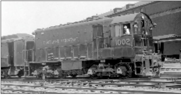
Portland Terminal Railway dieselized early, here ALCO HH600 diesel switcher 1002 is busy switching on August 16, 1937. Denver Public Library, Otto Perry collection, call number OP-14520.
