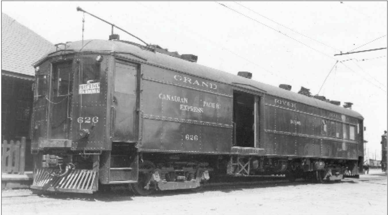
Express passenger car 626 was built by National Steel Car in Hamilton, Ontario in 1948. It was the last electric interurban car built in Canada. It is pictured here on May 1, 1948. The car was scrapped in Preston in 1957 when it was less than ten years old! CRHA Archives, Fonds Corley.
