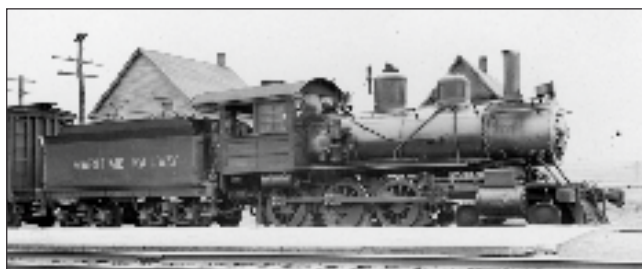
Maritime Railway No. 5 in service on that Nova Scotia coal road, note the unmodified flat valve gear and wooden cab! CRHA Archives
