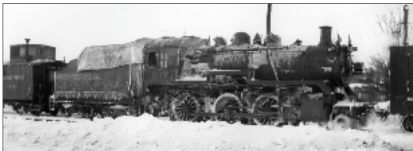
Canadian Pacific Railway 917 a D10g 'ten wheeler' built by the CPR in 1911 in snowplow service on January 4, 1947 at Tweed, Ontario. Al Paterson.
