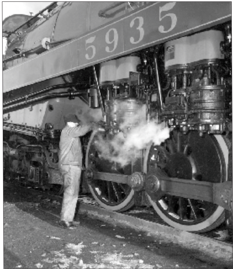
Oiling was a big part of keeping the steamers rolling. Here a fireman is oiling CPR Selkirk 5935 circa 1950. This locomotive forms part of the CPR historic collection at Exporail.
