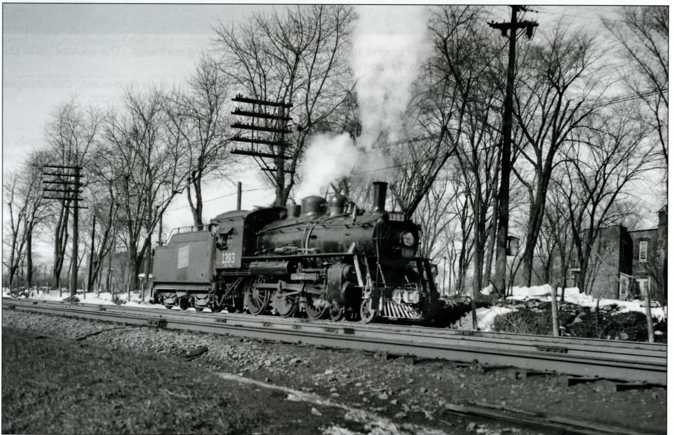
CNR 1393, an H-6-g 4-6-0 built by Montreal Locomotive Works in 1913, has just come off the Rawdon train at Gohier and is en route to Turcot Yards. Electric tunnel haulers took the passenger consist on to Central Station. Ernest Modler, Ronald Ritchie collection.
