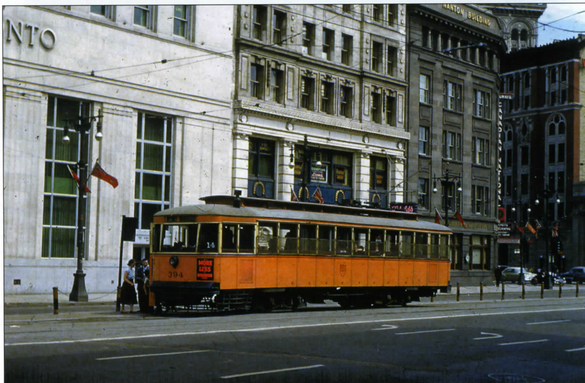
A clear 'blind side' shot of car 394 loading passengers on Portage Avenue on June 14, 1953. Built by the Winnipeg Electric Company in 1910, the blind side had 10 windows and the car was 4½ feet longer than earlier models. It was converted to one man operation in 1929. The front was modified to incorporate the 'Master Unit' look in 1937. Ronald Ritchie.
