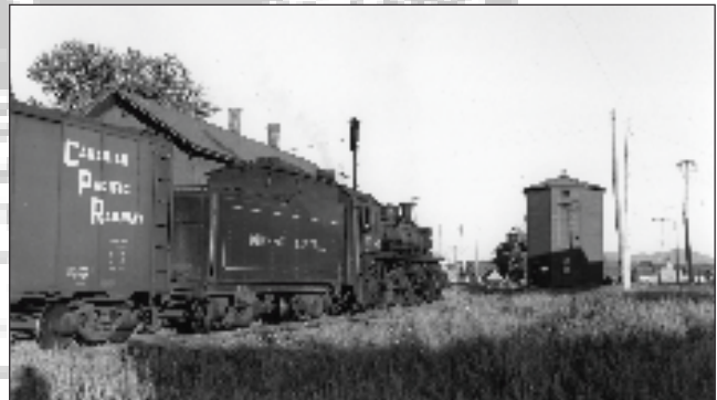
The lower quadrant train order signal indicates proceed as G2 2554 eases up to the octagonal water tank at Courcelles with mixed train No 24 on June 23, 1959. Eight sided water tanks were the norm on the QCR. Paterson-George, Stan Smaill collection.
