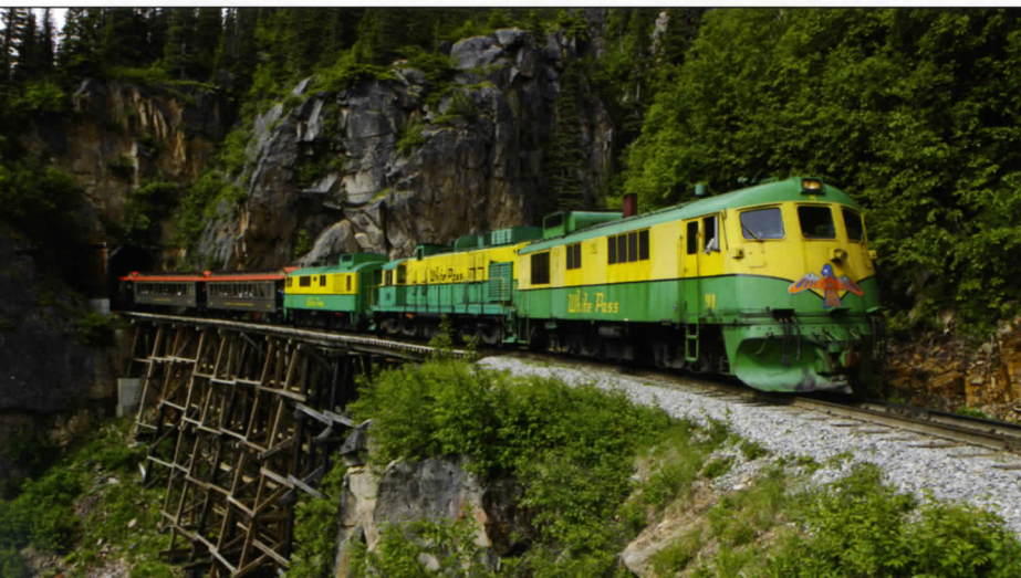
WP&Y GE 91 leads an Alco cousin and another GE on a southbound excursion train over bridge 15C. Number 91 was one of eleven units built by General Electric between 1954 and 1966. Interestingly, they featured a small 251 Alco diesel engine. Wouter Radstake.
