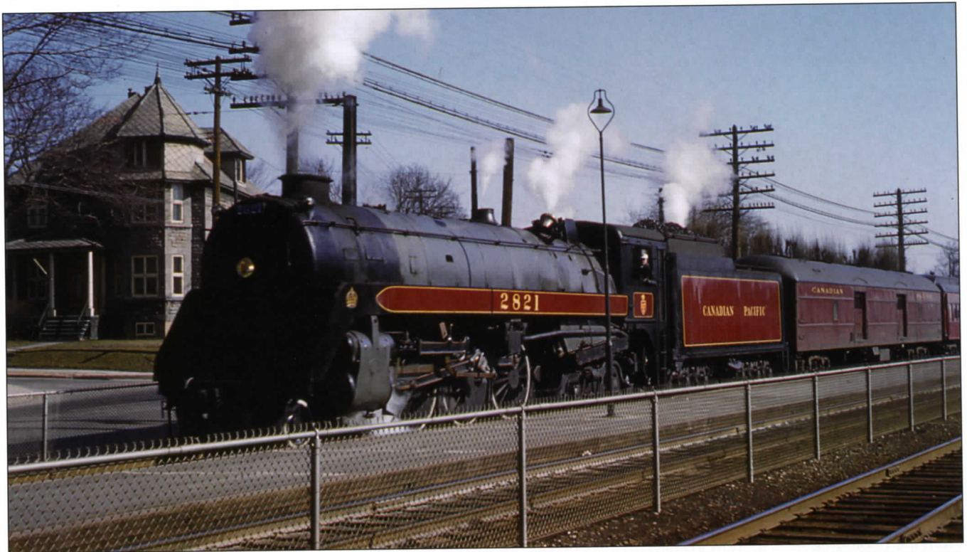
CPR H1c 4-6-4 2821 accelerates the morning local for Quebec City away from Montreal West Station on a beautiful spring morning circa 1954. The Gilbride mansion which stood at the corner of Brock Avenue and Sherbrooke Street appears prominently in this marvellous McGee image from the transition era. CRHA Archives, Fonds McGee.
