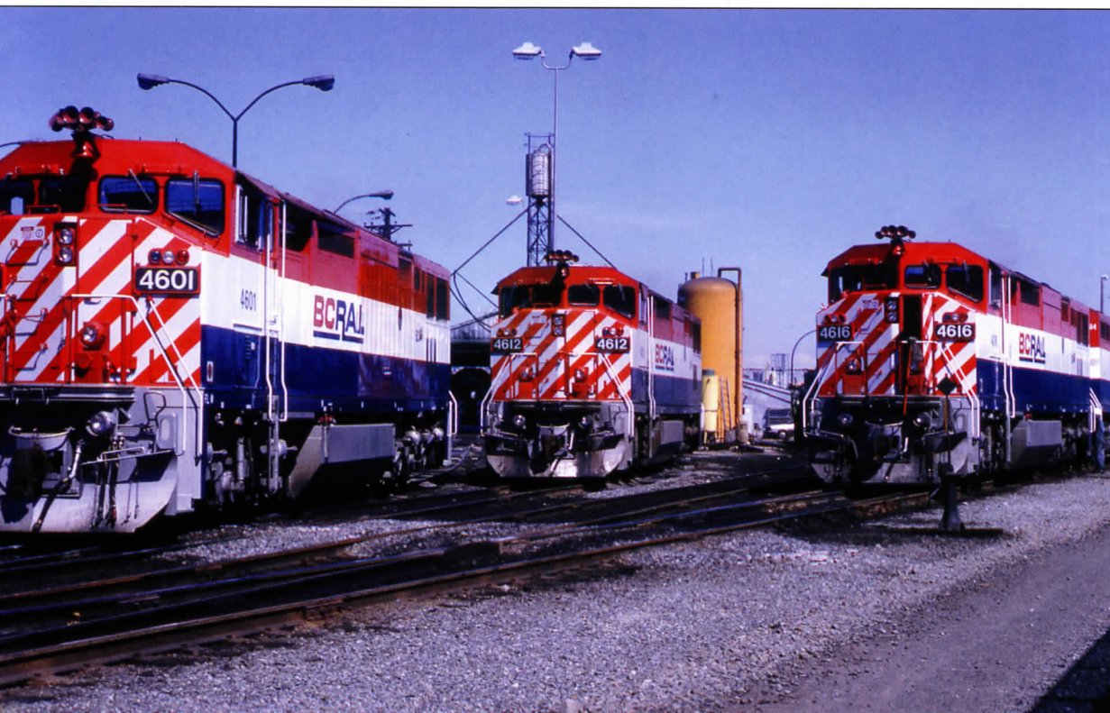
Three of the brand new fleet of General Electric Dash 8-40CMu's were caught by John C. Benson in North Vancouver on July 21, 1990. CRHA Archives, Fonds Bury, BCR1-111.
