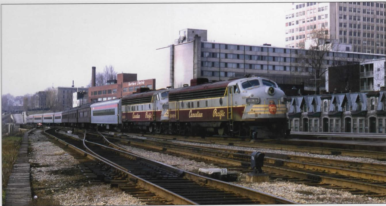
Arriving at CPR's Windsor Station circa 1969 with a Lakeshore commuter train is FP7 4068 assisted by a sister F coupled elephant style. It appears that the second unit has air brake problems necessitating the use of an additional unit for air brake control reasons. CPR 'A' units did not have nose MU equipment, so the second unit is on idle. Note the three heavyweight coaches in this mixed consist that includes 800 series coaches recently painted in the new CP Rail paint scheme.
