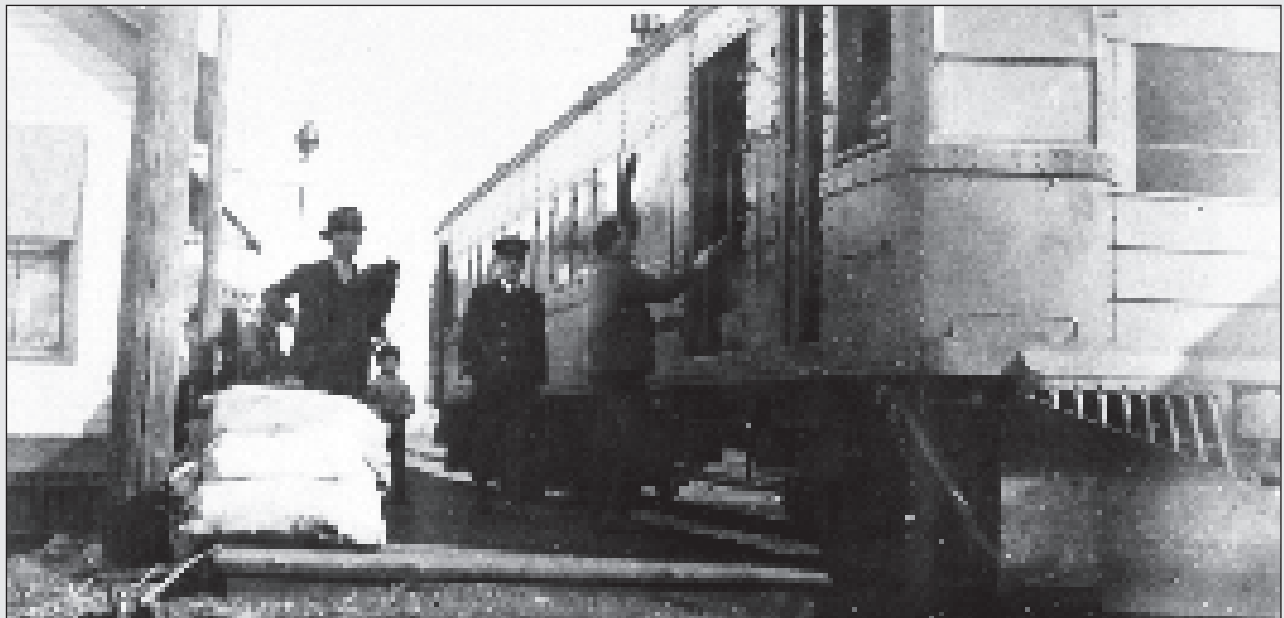
Great Northern gasoline-electric motorcar equipped with a snowplow doing station work at an unidentified location, probably in the 1930s. Royal British Columbia Museum Archives C-02193.
