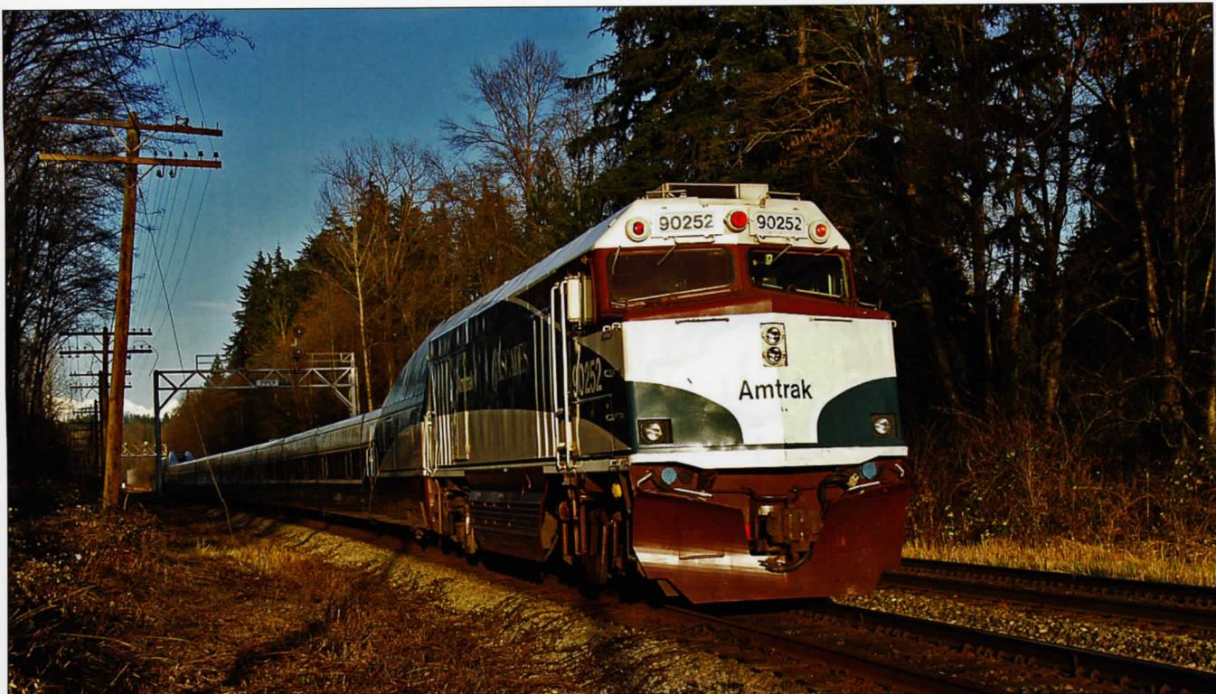
Operating on the rear of Amtrak's Vancouver-Seattle train 517, the five-digit road number indicates that unit 90252 is a demotored F40 control unit. A classic signal gantry of Great Northern origin beckons 517 through the control point known as Piper at milepost 148.1 of the CN New Westminster Subdivision on March 23, 2011. Ian Smith.
