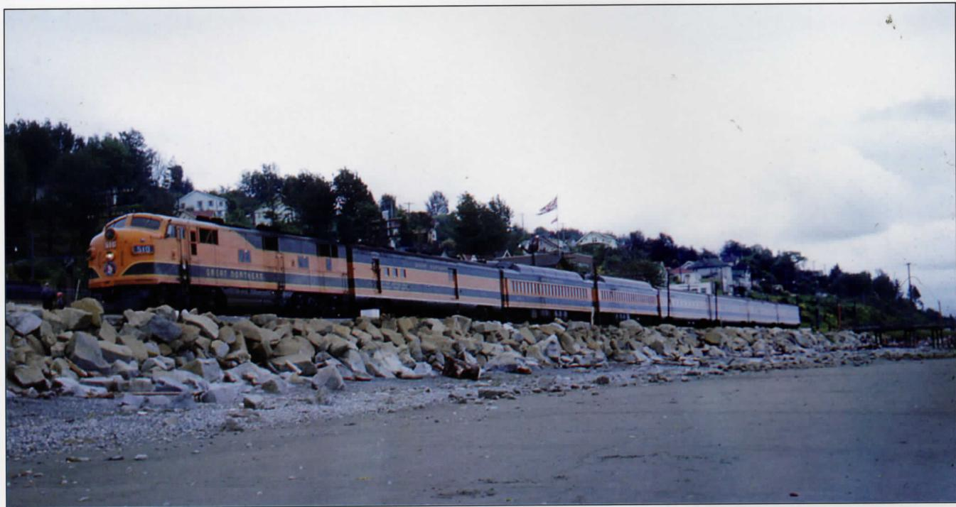
Great Northern initially dieselised its flagship streamlined passenger trains such as the *Empire Builder* and the *Western Star* with EMD E7's. After a short while in these services, the E7's were replaced with passenger F3's and F7's, which had better tractive effort and train heating capabilities. Bumped from her first job hauling the *Empire Builder*, Great Northern E7 510 has the *International* northbound for Vancouver at White Rock in the early 1950s. CRHA Archives, Fonds Bailey.
