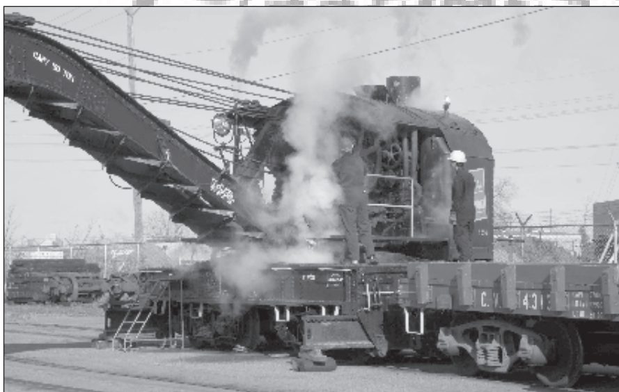
Bytown Railway Society fired up 4251 their 1919 50 ton Central Vermont operating steam crane. Don Evans.
