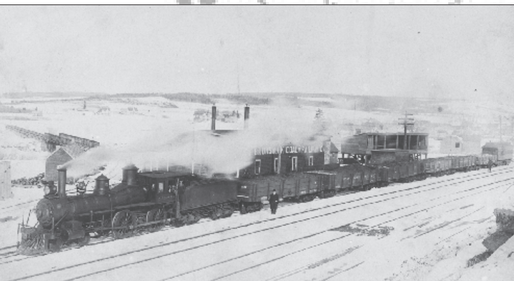
New Brunswick Coal and Railway American style 4-4-0 6 coming into the station at Norton, New Brunswick circa 1912; note the built up flat cars used for hauling coal from the Pennlyn coalfield to be picked up by the Intercolonial Railway and the wooden wedge plow parked behind the train. The bridge at the top of the photo runs north over the Kennebecasis River to Belleisle, Chipman and Minto. The other trackage is Intercolonial Railway's line between Moncton and Saint John. The wooden NBC&R's coal rack for coaling their locomotives; the wooden shop belongs to the NBC&R and survived into 1963. New Brunswick Museum and Archives 1967.81.21.5.; caption information Wendell Lemon
