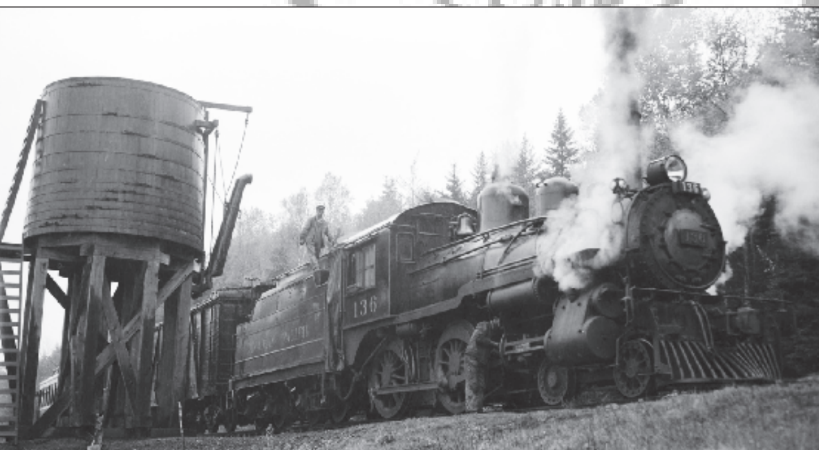
The Author's first trip to the Minto Subdivision was on May 25, 1949, 136 was the engine in service that day; 136 has just taken water at Perry, N. B. while a crew member checks the valve-gear. CRHA Archives, Fonds Toohey 49-263
