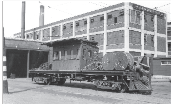
A trolley modelers delight! The origins of this car appear to be an 1896 double truck Hamilton Radial passenger car 15, it was converted to a freight motor in 1904, then to a line car in 1913. It had one controller for operation in either direction. It was assigned to the HSR in 1930 and had Baldwin MCB trucks installed c1933. It carried number 15 through to the end; this photo was taken at the car barn on July 11, 1949. CRHA Archives, Fonds Corley
