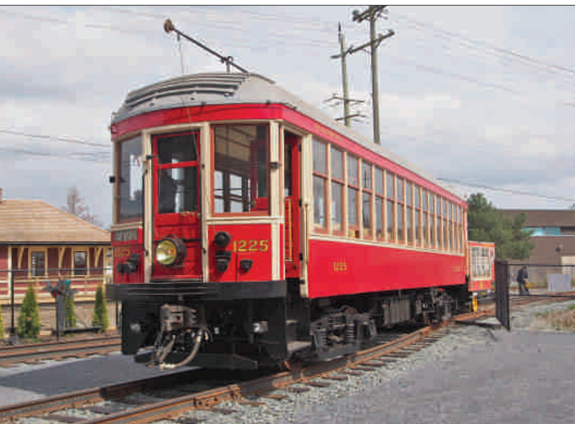
The Fraser Valley Heritage Railway commenced operations on June 22, 2013 when former BC Electric interurban car 1225 entered service between Cloverdale and Sullivan over former BCER trackage. A 600VDC motor-generator set was towed behind the car to provide the power (in lieu of overhead wires). Ian Smith
