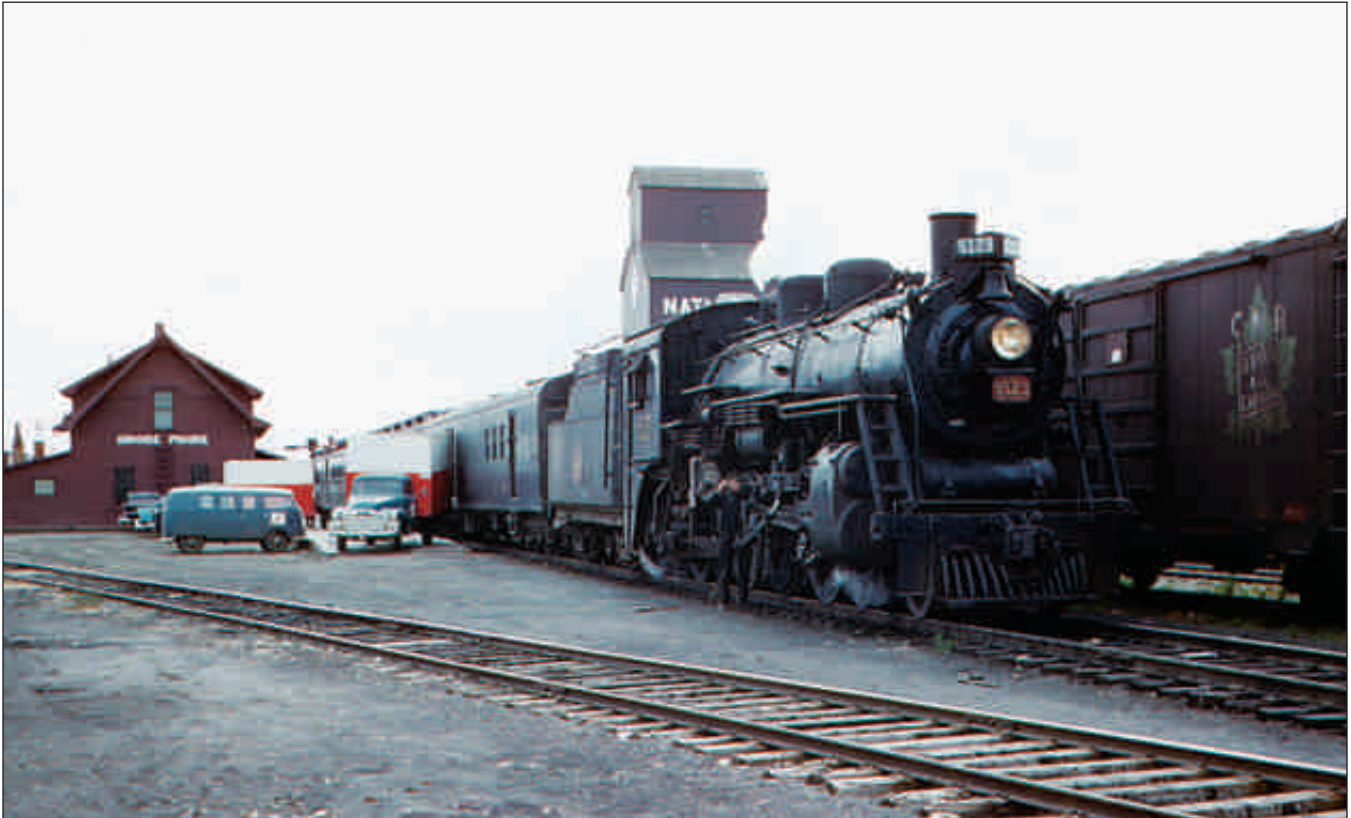
CNR 5123 was a 1919 Montreal Locomotive Works product. This 4-6-2 was classed as a J-4-d and was photographed at Grande Prairie, Alberta on NAR Train No. 1 in June 1959. C. Robert Craig Memorial Library, Fonds Kenneth F. Chivers
