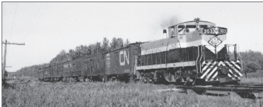
NAR GMD-1 locomotive 303 leads train No. 8, a through passenger train from Waterways to Edmonton, near Carbondale on September 12, 1964. The transition from steam to diesel has been firmly established but, with the exception of the CNR baggage car, the consist is similar to that found on this train a decade earlier. West Coast Railway Association Archives, Peter Cox collection
