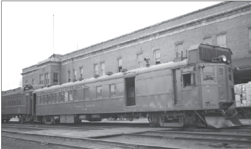
S&L trains interchanged with the CNR at New Glasgow, Nova Scotia; in 1949 the CNR was providing local passenger service with an oil-electric such as 15840 and coach pictured here. CRHA Archives, Fonds Toohey 49-293
