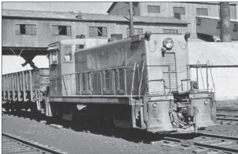
Acadia Coal 43, a GE 70 tonner works the wash plant at Stellarton, Nova Scotia in October of 1963. Jim Parker
