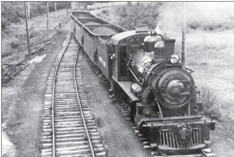
Maritime Railway 9 'coal hauling', it was a 2-6-0 built by Montreal Locomotive Works in 1910; after many years on other roads, it finally came to the MR in 1951 and worked for another 10 years. Library & Archives Canada, Fonds Merrillees
