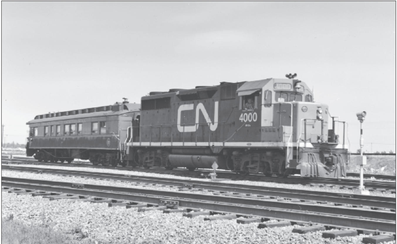
A small test train. Dynamometer car 69 represents the only load behind the GP35 unit which was being tested for train acceleration for possible use on the new GO Transit service. The train is sitting on the Montreal Yard diesel shop lead track waiting to go to Parsley Yard. Barry Biglow
