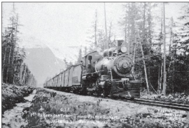
View of the first train from Prince Rupert at Mile 33 on June 14, 1911. The locomotive 103 was a 4-4-0 built by MLW in 1909 at a cost of $14,000. It later became CNR 377. The locomotive was shipped across Canada over the CPR and then by barge up to Prince Rupert. Royal British Columbia Museum Archives d00217
