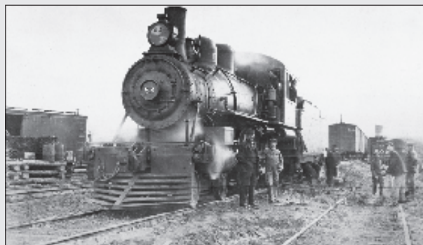
Locomotive 53 was a 4-4-0 built by Montreal Locomotive Works (MLW) in 1908. It was third to be produced in an order for 30 locomotives (GTP 51 to 80); it later became CNR 327. This photo was taken at Portage la Prairie, Manitoba. Glenbow Archives NA-3304-23
