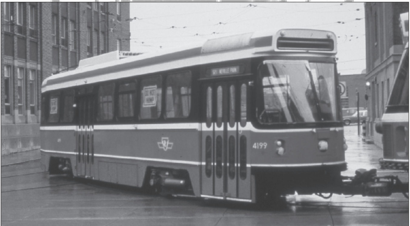
Brand new CLRV 4199 is being towed from Hillcrest Shops to the St. Clair car-house on Friday, November 20, 1981. In later years the couplers were removed and grey skirts added to the cars. J. D. Knowles, CRHA Archives, Fonds Wickson
