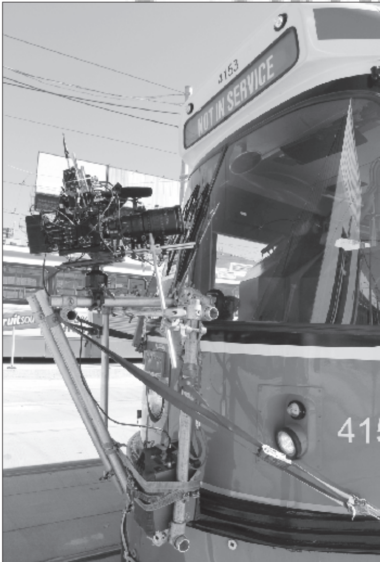
The IMAX camera mounting arrangement on the front of CLRV 4153, it is aimed to show a sequence of the operator of the car. Stephen Low Company
