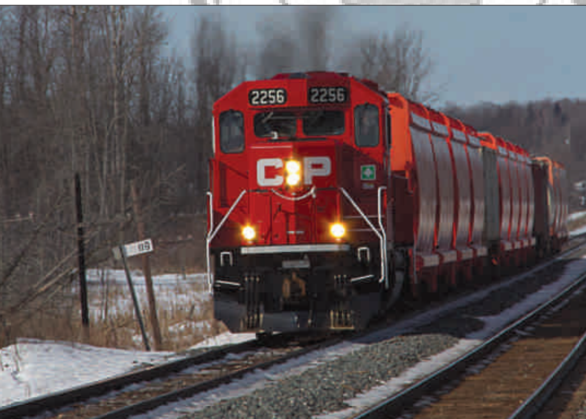
CPR GP20C-ECO 2256 powers a short 'DeBeaujeu turn' at MP119 of the CPR Winchester Subdivision on Monday, February 24, 2014. The new CPR 2200s are remanufactured using components from retired CPR Geeps. Robert Heathorn
