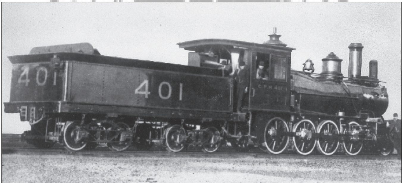
CPR 2-8-0 Brown SD Class 401 was built in the Canadian Pacific New Shops in Montreal in September, 1886 for service on the Big Hill. Within a few years they would be replaced by larger more powerful locomotives and reassigned to other duties. This turn-of-the-century (undated) photograph has a hand written inscription overleaf 'First hog to come to Fort William West in the days of the link and pin'. This view clearly shows the link and pin coupler pocket and the air brake hose. CPR Archives, 401
