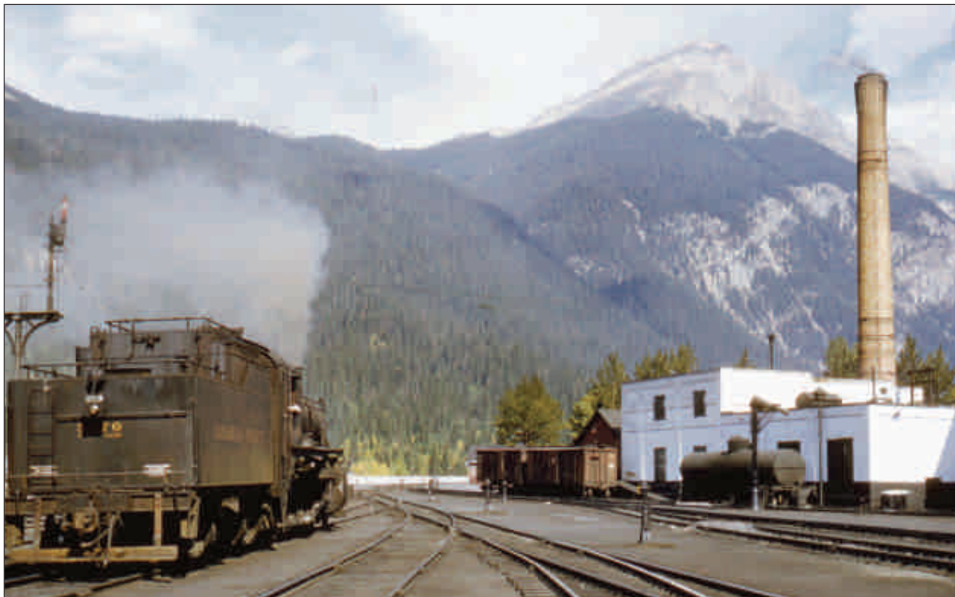
At the east end of Field Yard on September 17, 1951, Ron Ritchie found R class 2-10-0 5770 beside the power house facing the ageless mountains of Kicking Horse Pass. The cantilevered semaphore signals were fixtures at Field before target signals and CTC replaced them. R. S. Ritchie
