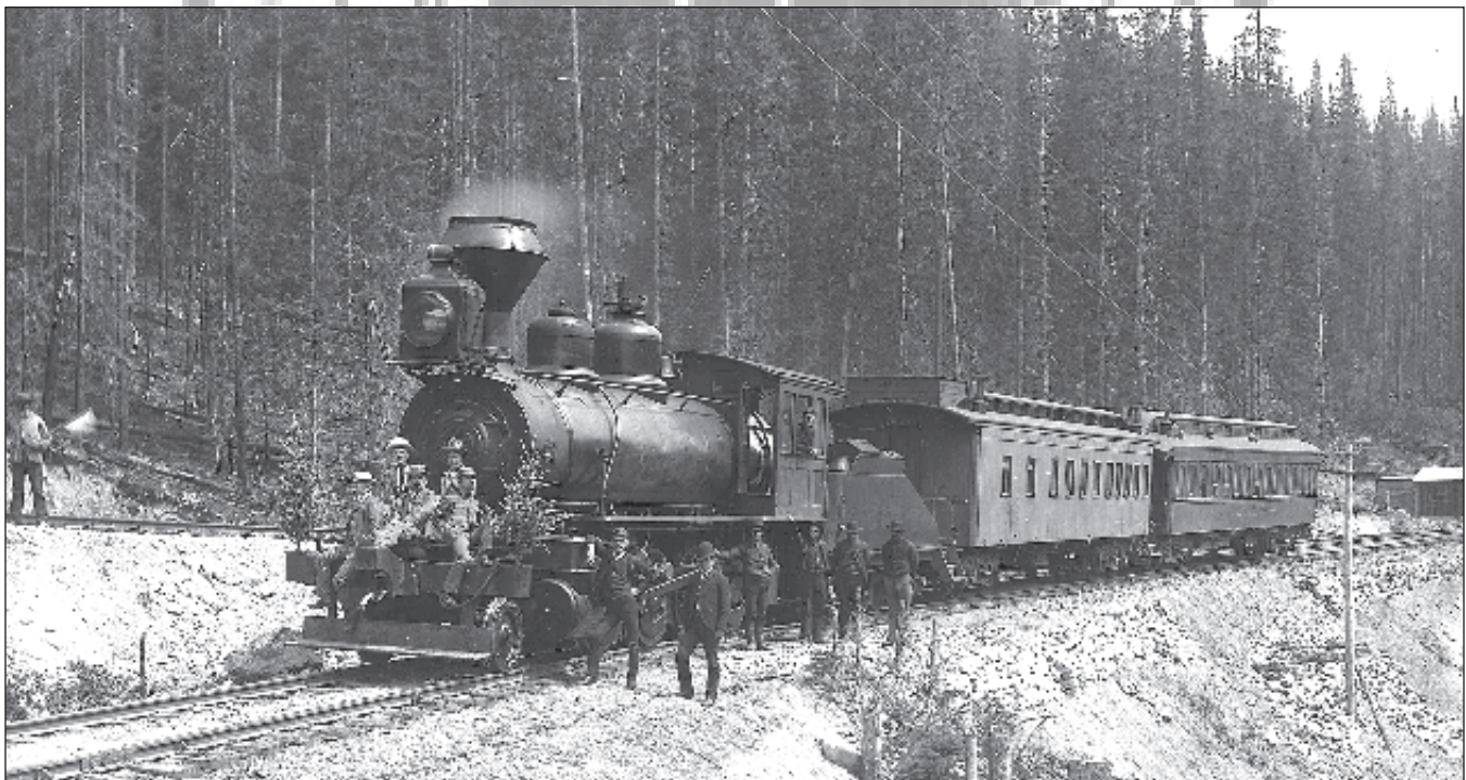
Another view of CPR Consolidation 315 coupled to two business cars which hosted a 'photographer's special' in 1889 or 1890 (conflicting dates). The location is safety switch 1, the run-off track is clearly visible in front of the locomotive. McCord Museum of Canadian History, view 2508
