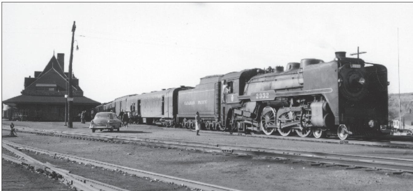
CPR 2332 was a G3d Class 4-6-2 built by MLW in 1926. It is pictured here handling The Gull at McAdam, New Brunswick on October 28, 1952. Ken McDonald
