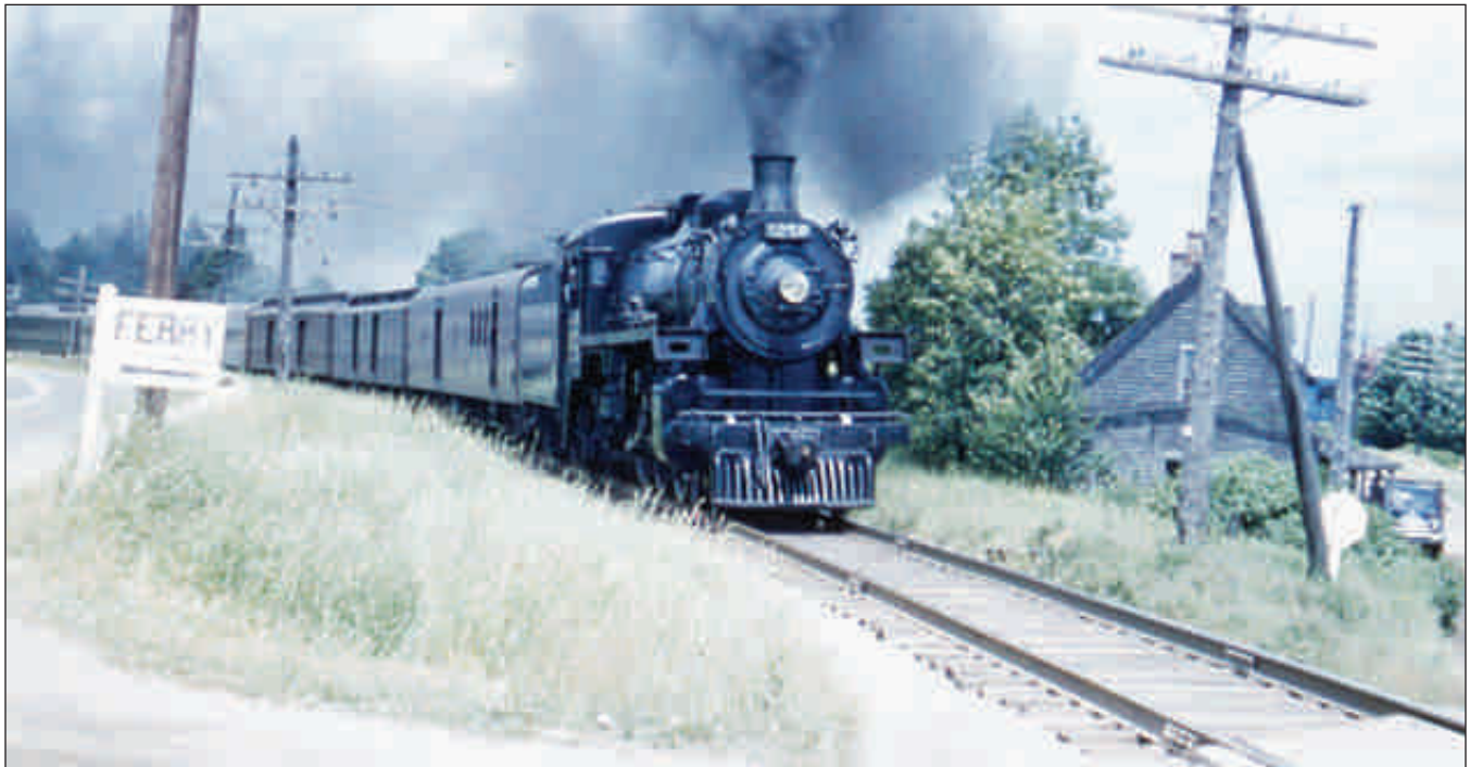
CPR G5 4-6-2 1258 has the eastbound Gull well in hand passing Westfield Beach, New Brunswick in 1956. On the CPR, The Gull was operated as trains 113 and 114 between Saint John, New Brunswick and Vanceboro, Maine until October 1959. Photographer unknown, Jim Simmons collection
