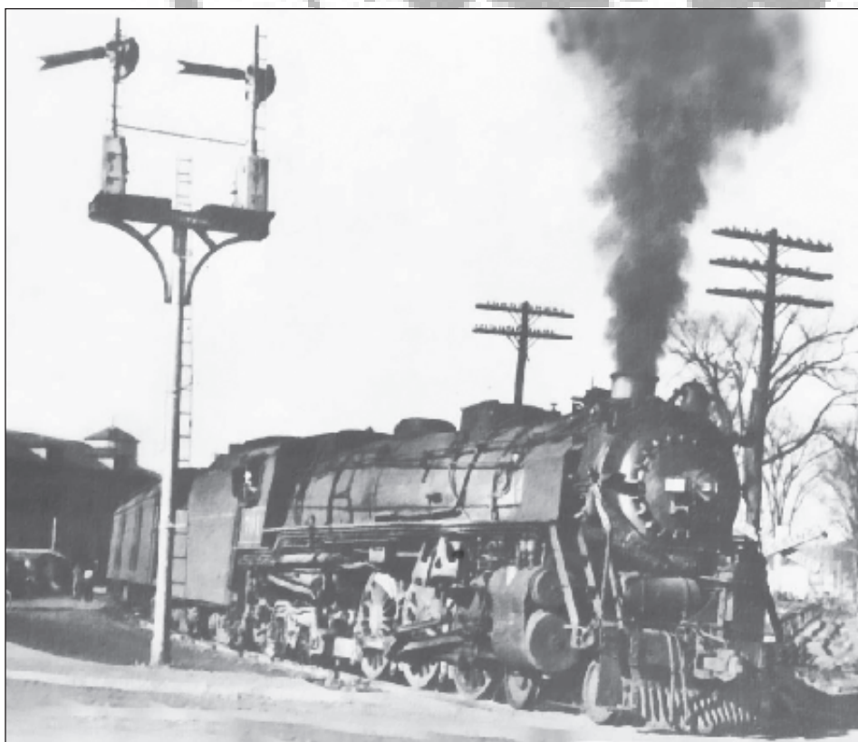
The 701, one of the Maine Central's big 4-6-4 Hudson Type locomotives which used to pull The Gull in the later steam era. Location and photographer unknown, Jim Simmons collection
