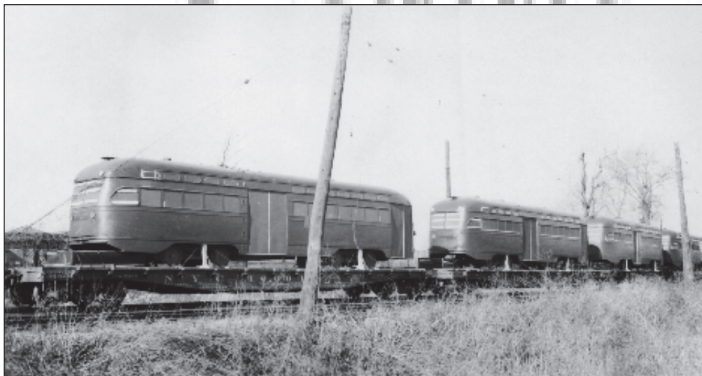
Body shells for TTC's 4500 - 4549 series (Class A8) leave St. Louis Car Co. in 1950. CRHA Archives, Fonds Bailey
