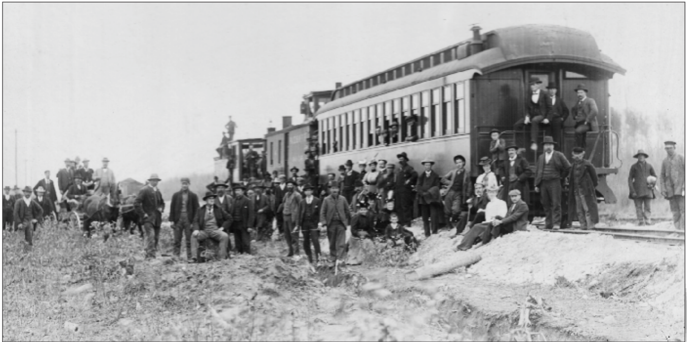
Labelled as the first train into Swan River, this appears to be an excursion – possibly for land sales purposes – that followed on the heels of the construction train in October 1899. The side door caboose appears to be lettered for the LMR&CC and supports its marker light upon the side of the cupola as was the standard in the nineteenth century. Source: Swan River Historical Museum
