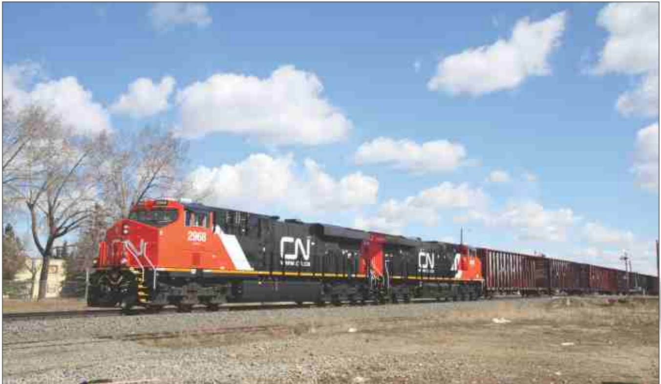
About six-million dollars worth of new diesel power in the form of brand new CN ES44AC's head west at Stony Plain, Alberta, on their maiden trip back on April 15, 2015. The two big GE's develop 8800 horsepower, more than a five unit lashup of fifties era first generation diesels! John A. Rushton
