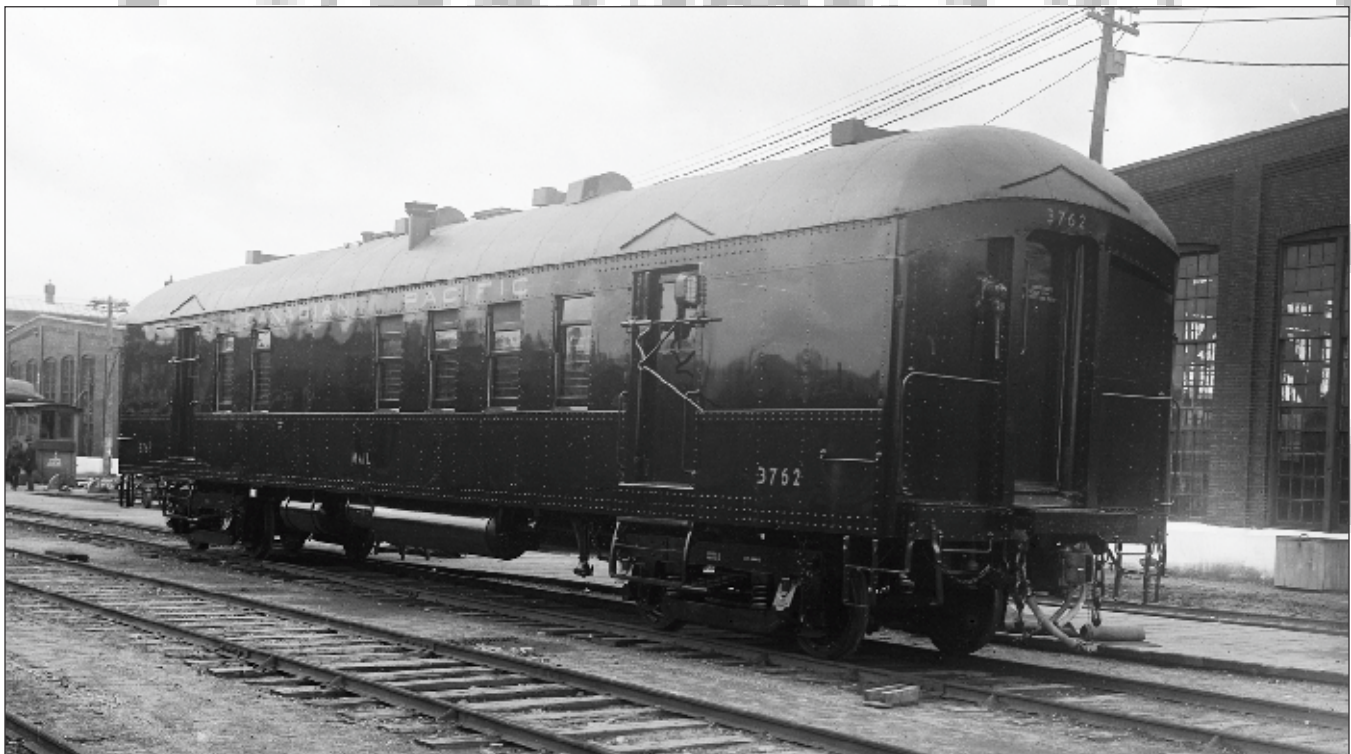
Mail car 3762 after modifications was riding on six wheel trucks and the Burnett roof had been replaced with a more standard wooden monitor roof, canvas covered. CPR Archives 201241
