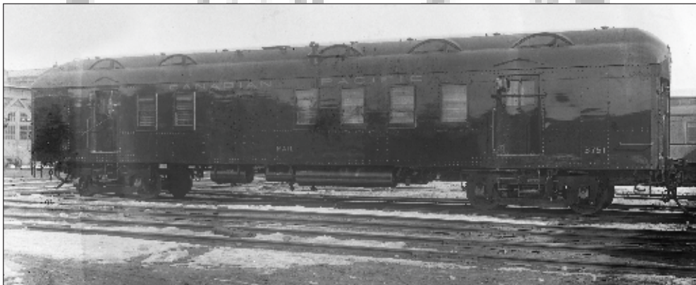
Mail car 3762 is part of the 1917 order with changes made by C.W. Van Burin to the Burnett design. The steel side plating is horizontal rather than vertical and the roof is the turtleback or Harriman style, which would replaced the Burnett roofs between 1919 and 1950. CPR Archives 201241
