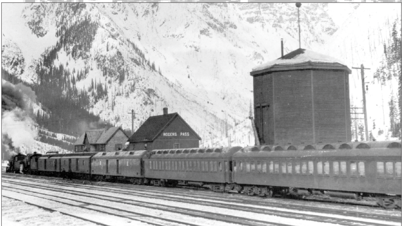
This is the CPR's premier train No. 2 the Imperial Limited, at Rogers Pass in October 1916. The steel Burnett cars can be easily spotted by the roof dormers. Doug Phillips collection
