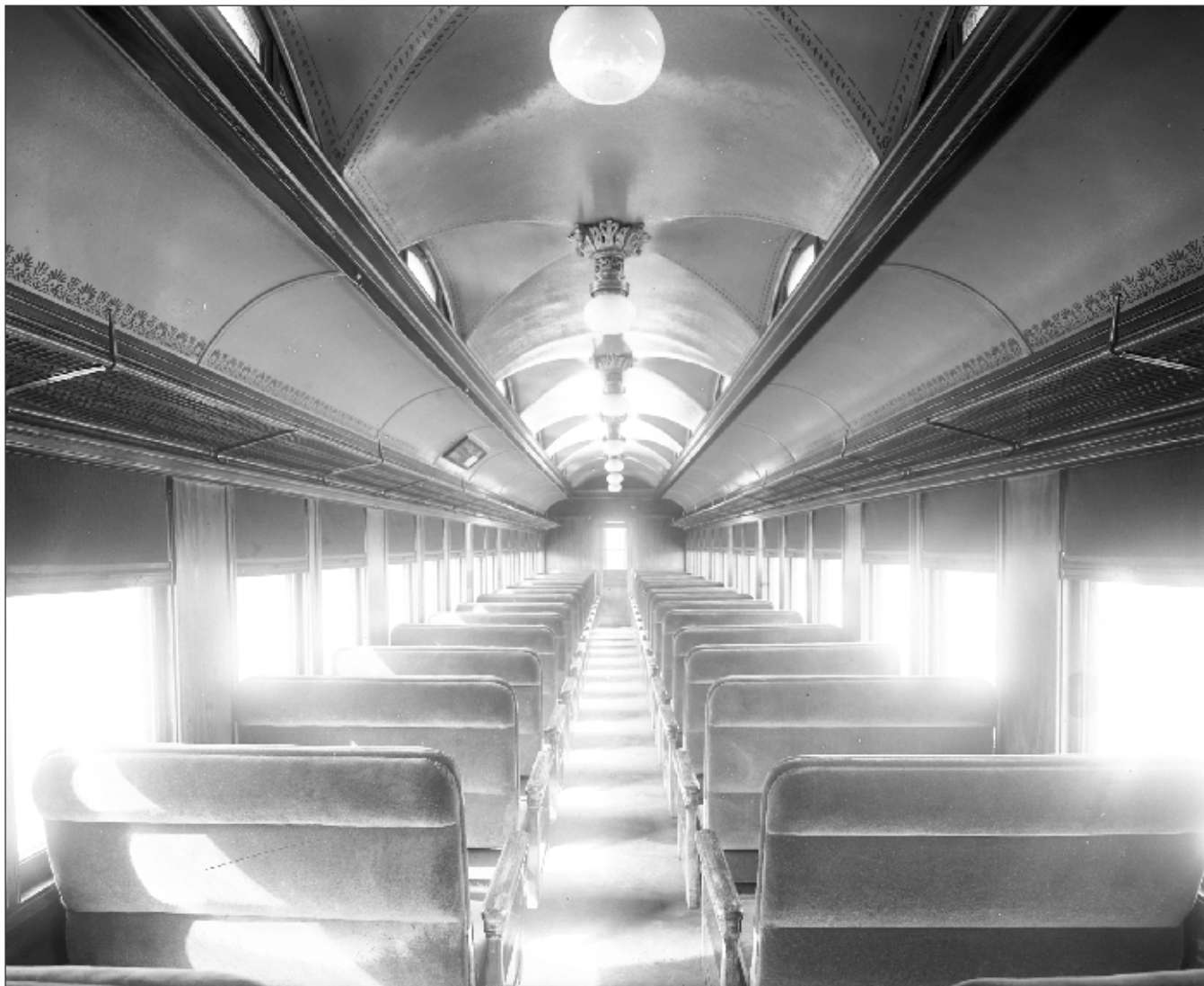
The 'Empire Deck' ceiling is evident in this photo of a first class coach. CPR Archives
