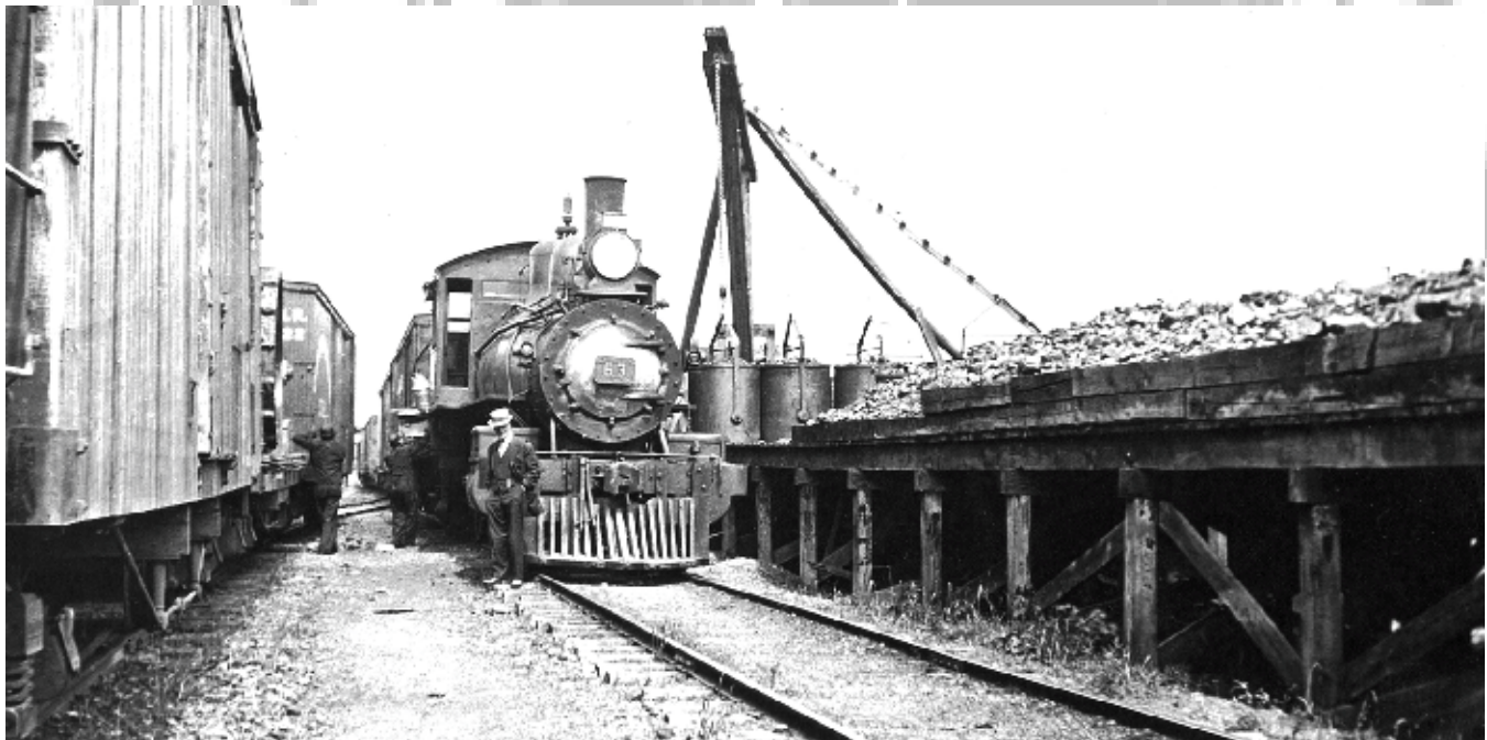
In later years circa 1915, Canadian Northern Railway 63, a Class B-2-A 4-4-0 built by Rhode Island in 1885, was photographed at Swan River, Manitoba. It came to the CNoR second hand from the AT&SF, it later became CNR B-2-a 213 and was scrapped in 1920. Ralph Friske collection, capiton information Don McQueen.
