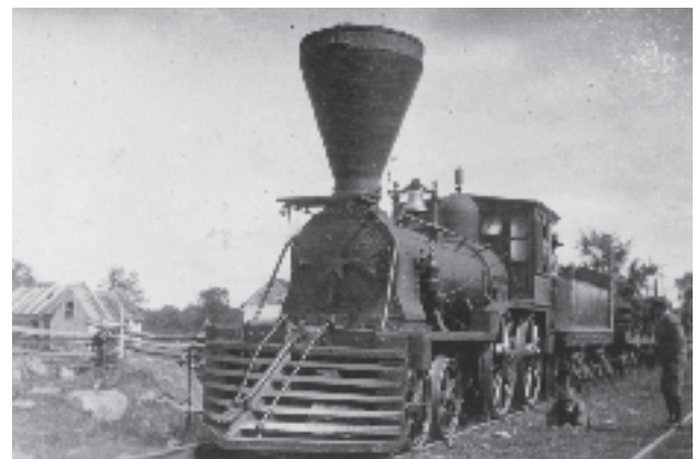
Carillon & Grenville Railway Steam Locomotive; The "Ottawa" wood locomotive, c. 1890. Exporail, Charlotte M. Owens Collection
