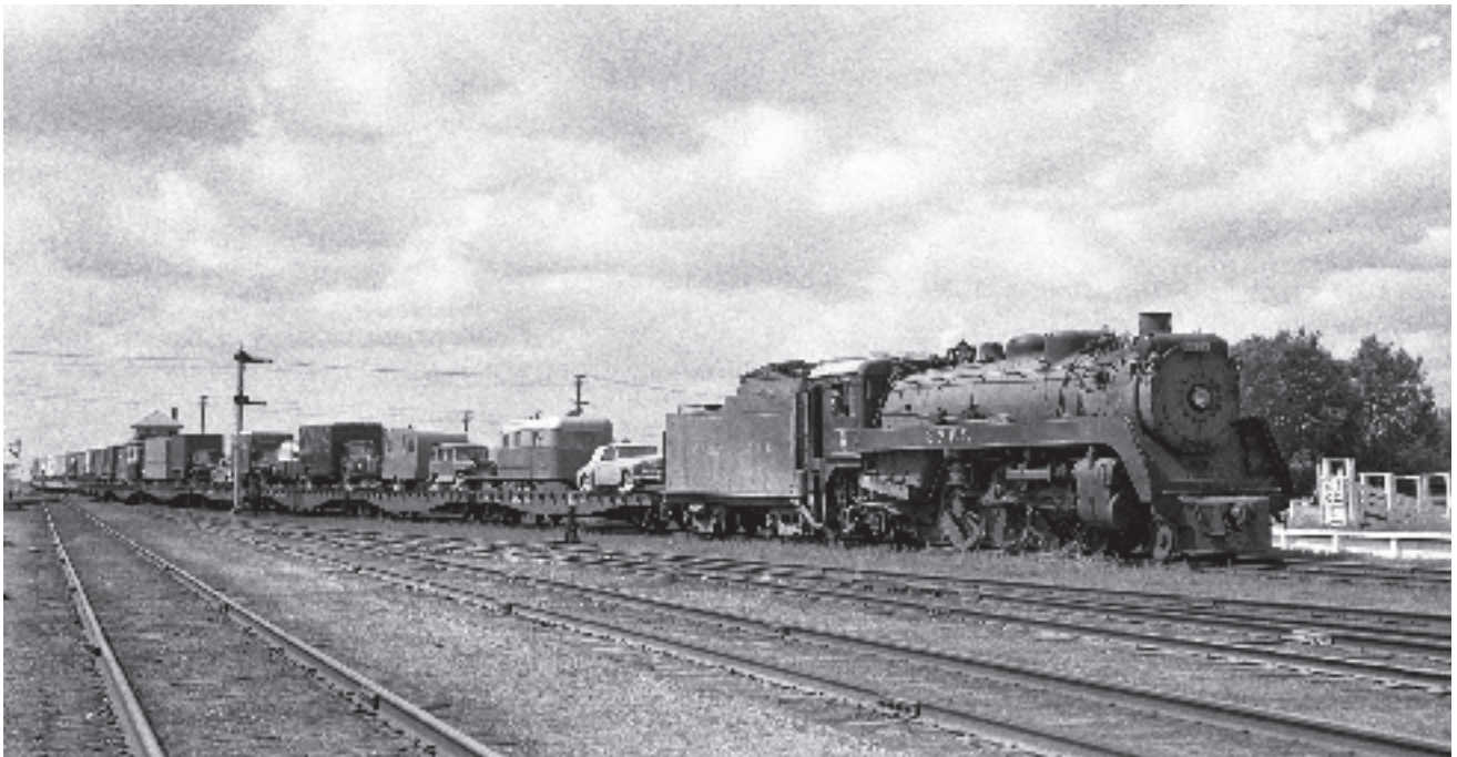
Canadian Pacific Railway's Class G3E 4-6-2 2363 (Canadian Locomotive Company , November 1938) eases a Royal American Show special into Brandon, Manitoba in 1950. Lawrence Stuckey, James Brown collection
