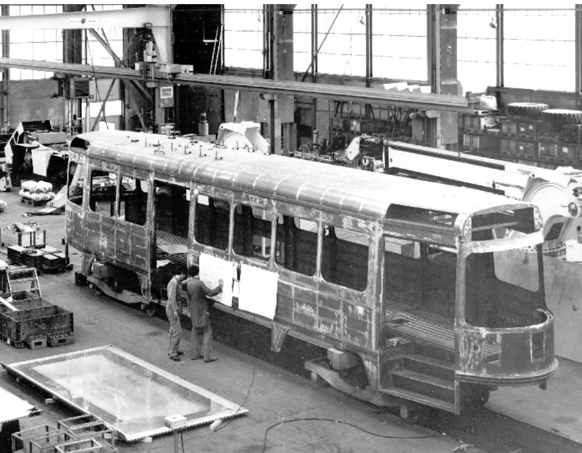
One of the ten prototype TTC streetcars under construction at Schweizerische Industrie Gesellschaft (SIG) in Neuhausen, Switzerland. UTDC, Ted Wickson collection
