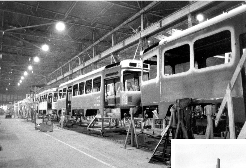
New TTC streetcars being manufactured at Hawker Siddeley's plant in Thunder Bay, Ontario in the fall of 1978. Hawker Siddeley, Ted Wickson collection
