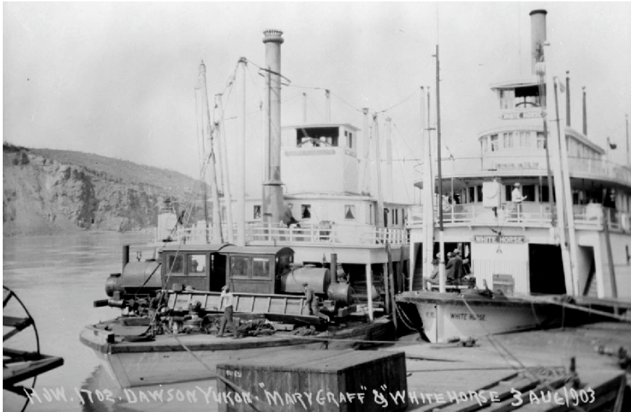
Two locomotives c/n 1167 and c/n 922 in their new configuration are on board the sternwheeler Mary Graff en route to Coal Creek, Yukon Territory in 1903. Library and Archives Canada, 3300370
