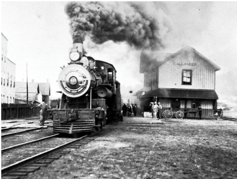
GTR 4-6-0 421 puts on a fine head of steam as it pulls into the Callander, Ontario station. Built in 1907 at the GTR shops, it was renumbered 1021 in 1910. Municipality of Callander
