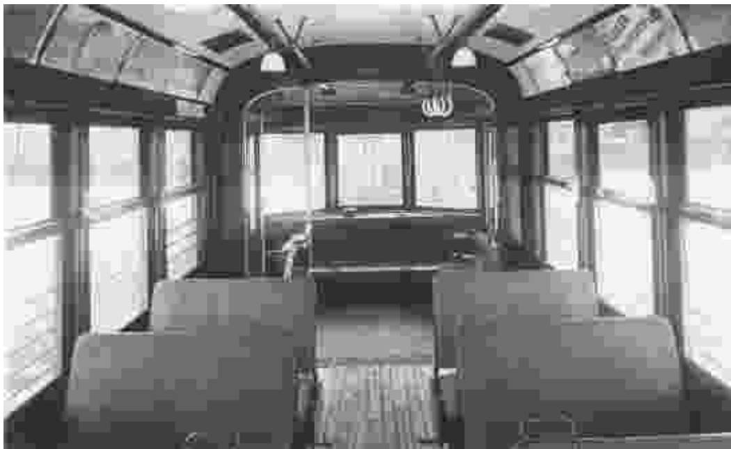
This is car 410 with the rear set of controls 'boxed over' and the conductor's position installed. CRHA / ACHF Exporail Archives, Corley fonds
