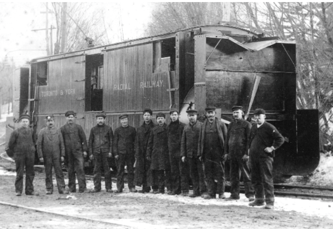
A dozen Toronto & York workers pose beside No. 90, a Ruggles 1904 rotary snow plow. There is no information as to when and where. CRHA / ACHF Exporail Archives, Paterson fonds
