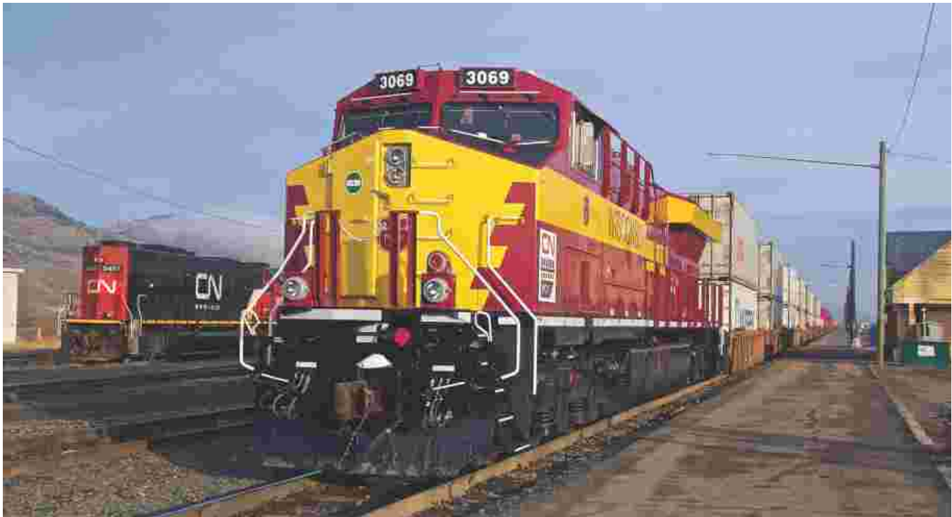
CN 3069 is the Wisconsin Central painted 'heritage' unit and is at Kamloops Junction, BC with a westbound stack train on November 27, 2020. CN 3069 is a GE ET44AC built in 2016. Russ Grycan
