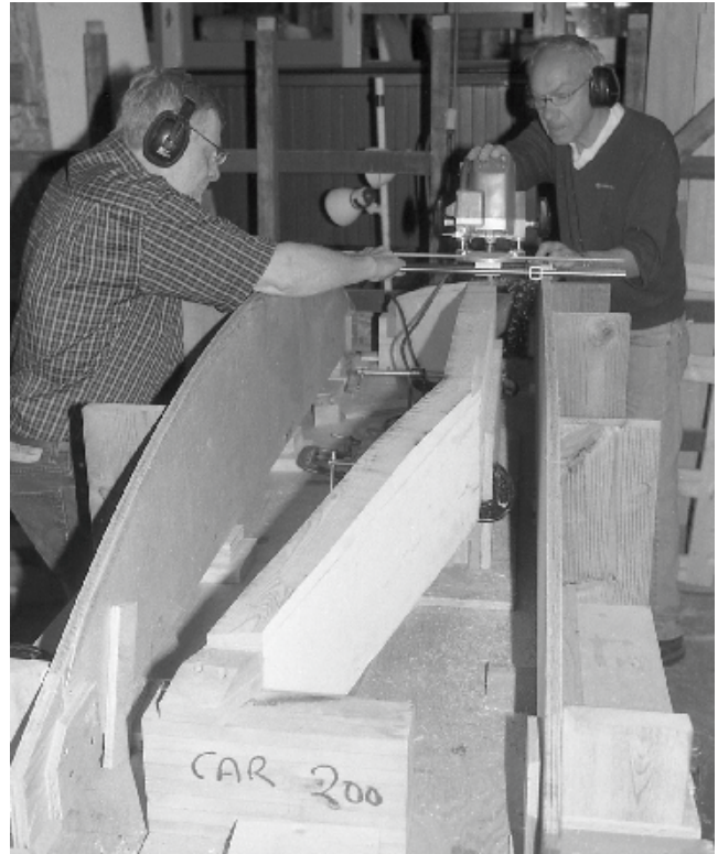
Barry Wiens and Allan Muir use a router mounted on a mobile wagon to cut the Saskatoon 200 end header roof curve dictated by the enclosing jig. (Don Scafe)
