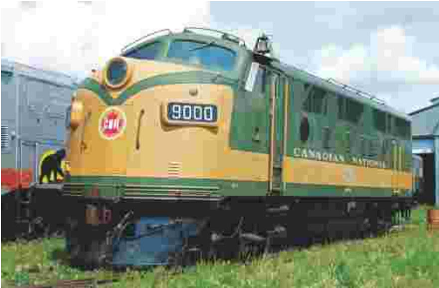
CNR's first road diesel F3A 9000 was built in 1948. It is preserved at the Alberta Railway Museum in Edmonton, this photo dates from 2010. Steve Arnot
