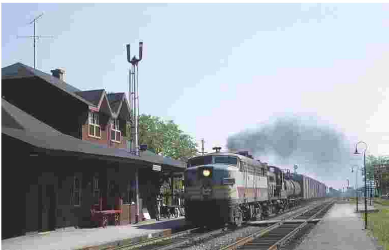
Changes at Winchester. Over the years the bay window on the second floor of the station was eliminated and insul-brick covered its sides. The most telling changes were on the rails with the switch from steam to diesel symbolizing the technological changes sweeping Canadian transportation. In 1965, a westbound freight rolls through the town behind FA-2 4044 and RS-3 8426. WR Linley
