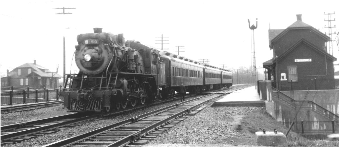
Later in time, circa 1954, we find CNR X-10-a 4-6-4T 50, the last of the class, at Dorval. Changes have come to CNR Dorval as the Cote de Liesse road underpass has now replaced the level crossing seen in the previous photo. Al Paterson, Smail collection
