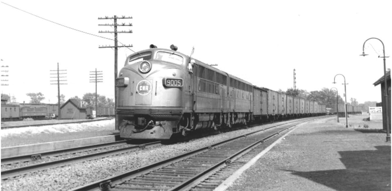
Diesels came to CNR main line freight service in the late 1940s with the delivery of American built General Motors F3 diesels in the 9000 series. Circa 1950, CNR F3 9005 powers an extra west at Dorval. The 9005 was involved in a serious collision which resulted in her being rebuilt as GP7m 4824 in October 1958. Al Paterson, Smaill collection
