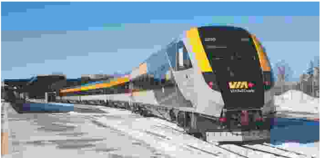
VIA's new trainsets are equipped with standard couplers on the noses of the locomotive and cab-control cars only; intermediate cars are semi-permanently coupled using proprietary connections. This is the normal arrangement for the Venture trainsets, and provides fully ADA-compliant passage between cars for passengers with reduced mobility. Amtrak Midwest is currently the only Venture customer to specify standard couplers throughout.
