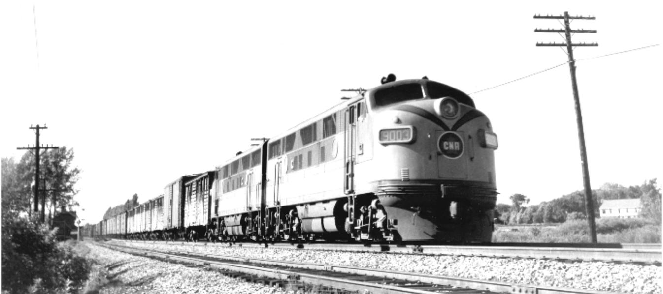
A block of cattle cars, spliced by a lone forty-foot steel boxcar, is marshalled ahead of five refrigerator cars on the head end of CNR manifest freight No 404 running as Extra 9003 East. The yellow paint has replaced the gold / bronze livery that CNR 9003 carried when delivered in 1948, making this, an early fifties view taken east of Dorval. Al Paterson, Smaill collection
