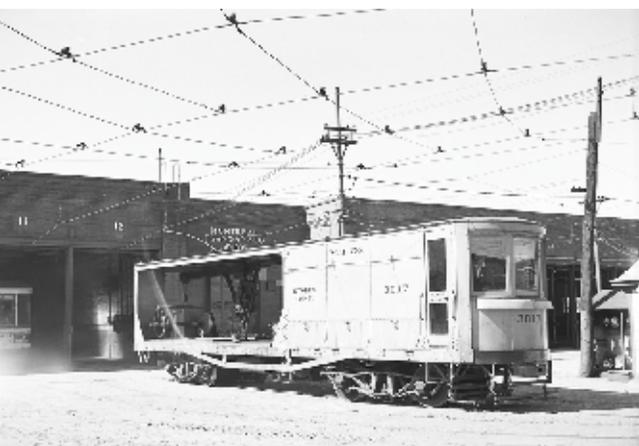
Officials at the St. Denis Division brought out some specialty cars for viewing by NRHS delegates. This photo shows MTC 3017 'Stores Car' which was used to transport tramway parts between Youville Shops and the various divisions. Note the wheel-set attached to the boom at the rear of the car. CRHA / ACHF Exporail Archives, Fonds Toohey 51-652
