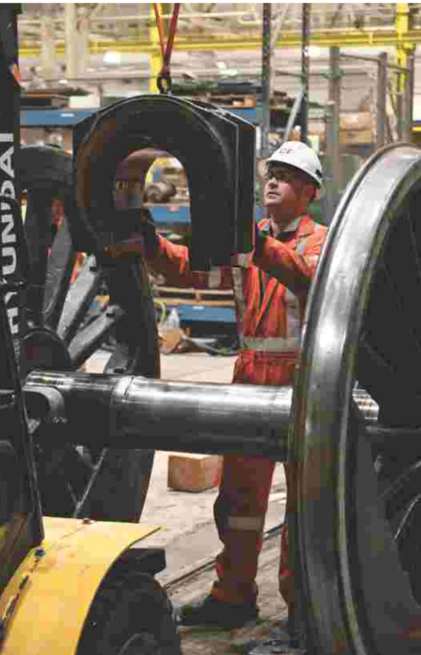
Jonathan Morris lifts a journal box off one of 2816's drivers during preparations for the conversion to oil lubrication.
