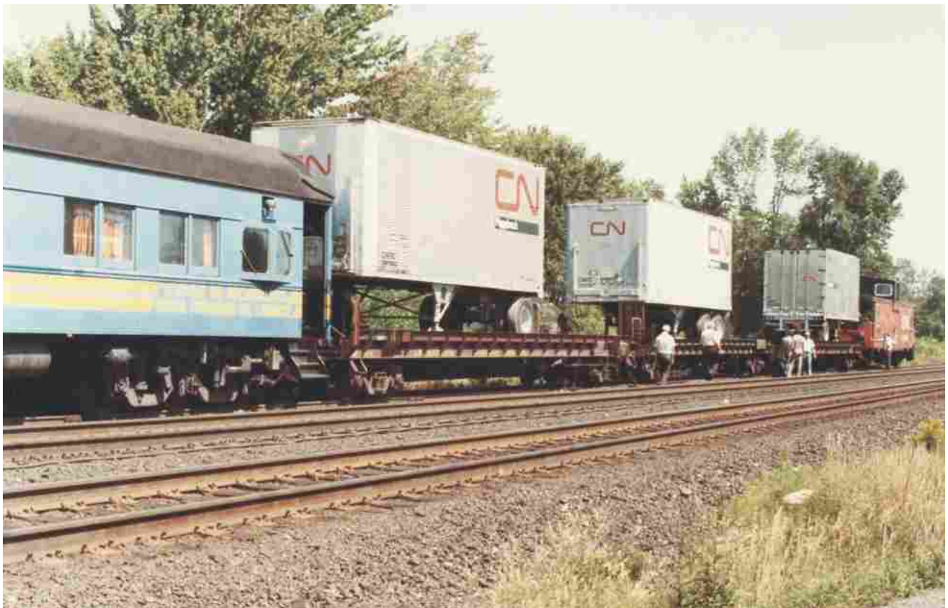
A very early test of constant contact side bearings on TOFC flat car trucks. The CN research test car, a converted heavyweight passenger car, is monitoring the flat car ride quality on a test trip to Ottawa. Kevin Day
