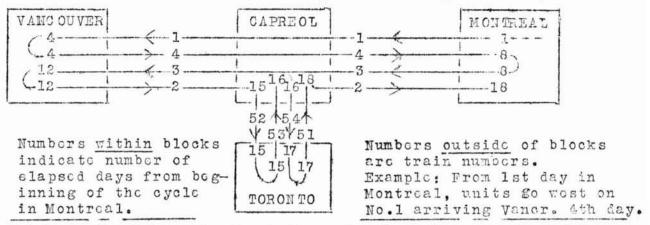
which is shown here in chart form, involves the use of eighteen sets of diesel-electric locomotives. After performing the cycle, at the end of eighteen days, each locomotive set has completed 12,825 running miles, and lays over for more than twenty two hours in Montreal for inspection, before performing the cycle again, by leaving Montreal on No.1 on the nineteenth day.
