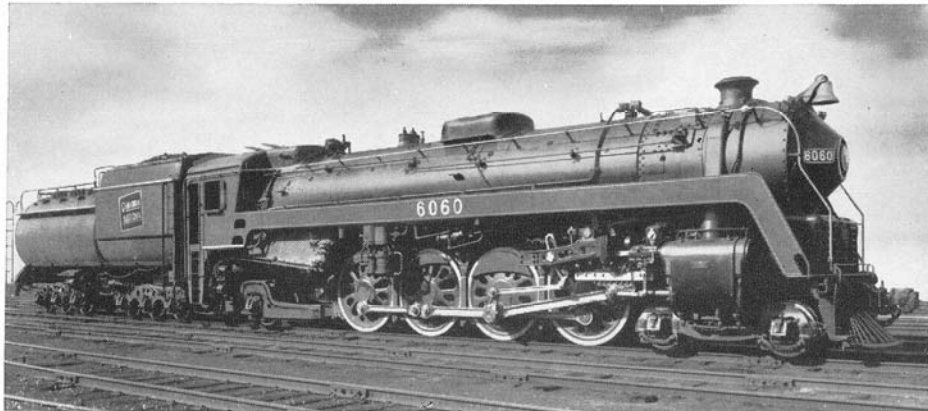
This Mountain type locomotive (Class U-1 — Road Numbers 6060 to 6079) was built for Canadian National Railways by the Montreal Locomotive Works in 1944.
