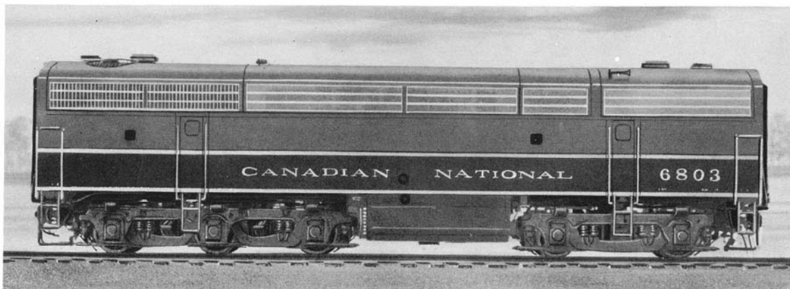
This Diesel-Electric Passenger locomotive (B unit) (Class CPB-16 — Road Numbers 6800-6805) was built for Canadian National Railways by the Canadian Locomotive Company in 1955.
