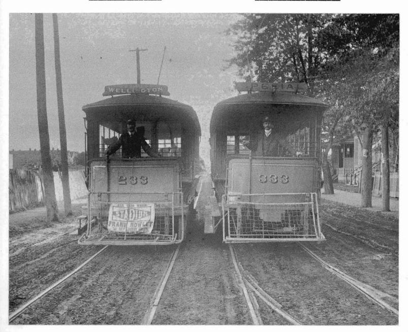
AROUND 1905, two M.S.R. open cars, 2nd No. 233, Lot 10, left, and No. 333, Lot 8, right, were lined up on adjacent tracks, both facing east, for a photographer at Beresford and Wellington streets, in Point St. Charles. No. 233, on the regular Wellington route, has a sheathed blind side, while No. 333, a special car, has wire screening only. Both cars were scrapped by the M.T.C. in June, 1924.
